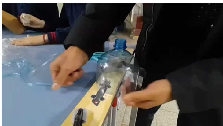
Figura 9. Obtención de hilos a partir de botellas de PET. Figure 9. Obtaining threads from PET bottles.
