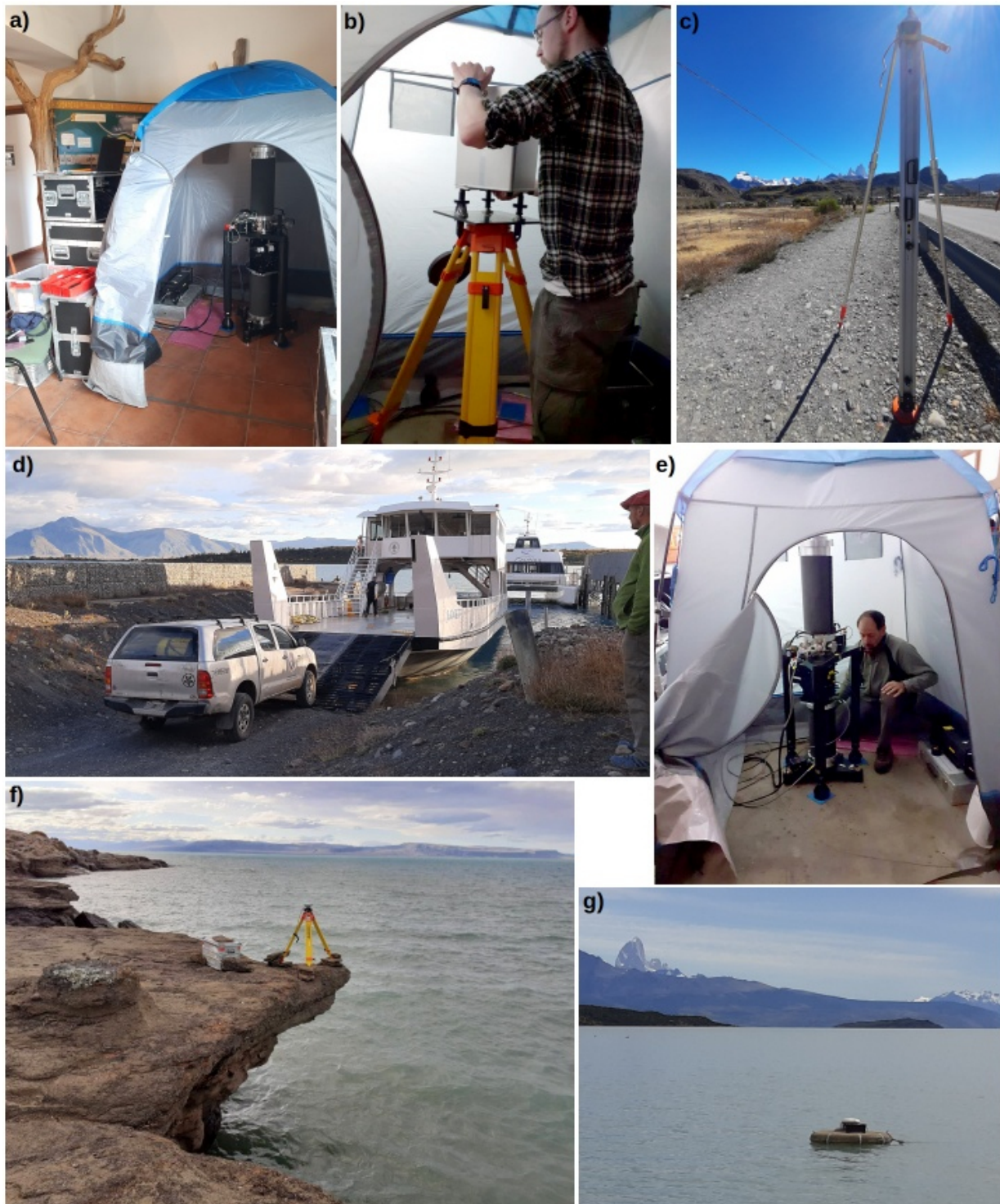
Figure 3. Impressions from the fieldwork in southern Patagonia. a) FG5-227 absolute gravimeter in operation at site CHT; b) Relative gravimetric observations for gravity gradient determination at GPM; c) Levelling at site CHT; d) Transportation of the gravimeter equipment to the remote CRS site; e) Installation of the FG5-227 gravimeter at site GPM; f) Reflectometric water-level monitoring in Lago Argentino, close to FTE site; g) GNSS buoy operated in Lago Viedma at HLS site. All pictures were taken during the 2022 campaign, except g) (2020).
