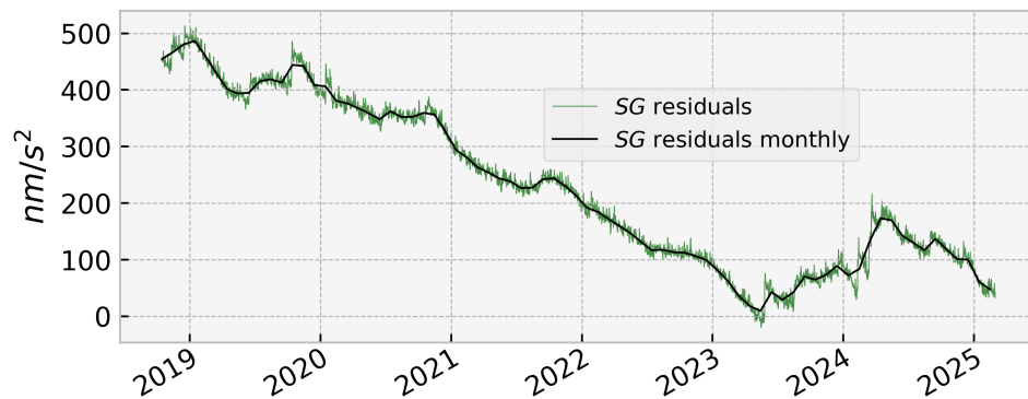
Figure 1. SG038 gravity residuals recorded at AGGO. In green, gravity residuals with 1-hour sampling. In black, the same time series down-sampled to monthly resolution after applying the moving average window.
